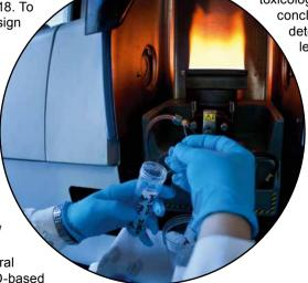
Eurofins BioPharma Product Testing is able to perform screening of more than 35 inorganic elements by ICP technique and is equipped with two kinds of LC-MS for organic non-volatile
